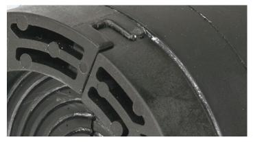
press plate with form-fitting connection
